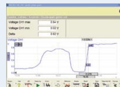
Oxygen Sensor Test measures low voltage signal
